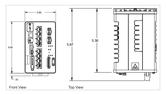
**Figure 2.** Cisco Catalyst IE3200 dimensions
