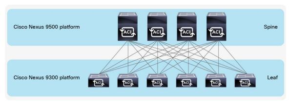
**Figure 2.**Spine-Leaf Architecture using Cisco Nexus 9300 and 9500 Switches
